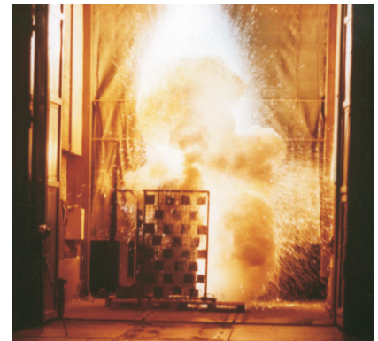
PICTURE: NorPower 5000 is arc-tested at the test laboratory
