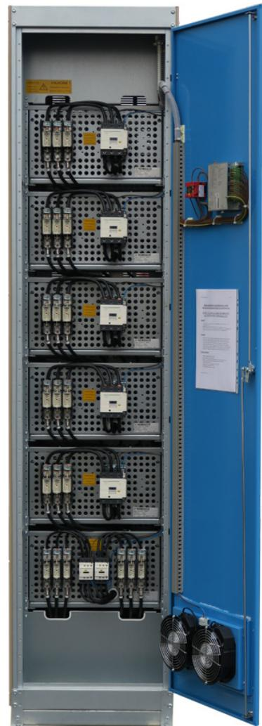
The system is very modular, since each cassette consists of all the components, namely capacitors, fuses, contactor and blocking inductance. Compensation system is manufactured using 3-phase condensators. Discharging resistors are included discharging condensator below 50V in 50sec after disconnection. Condensators are gas insulated and self-healing type.
